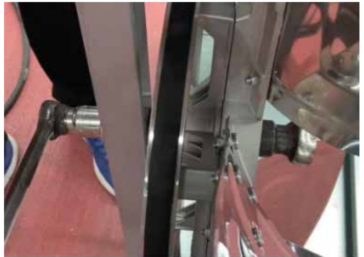
Figure 11. Propeller Shaft Adjustment.
