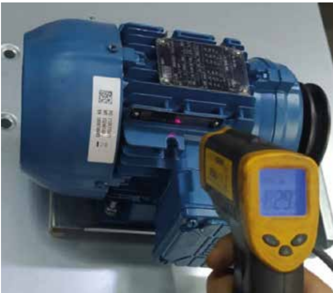
Figure 10. Measurement of temperature in the motor with a laser thermometer.
