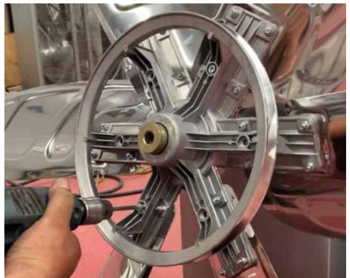
Figure 12. Adjustment of blade-to-hub fastening bolts.
